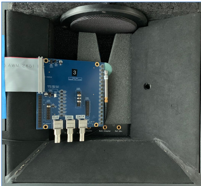
Figure 5. The microphone array test fixture located in the acoustic test box.
